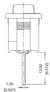
T(Quick connect tab:Thickness of 0.8mm)
