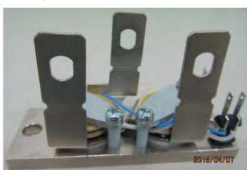
Pressure contact design – no wire bonds, no solder fixation
